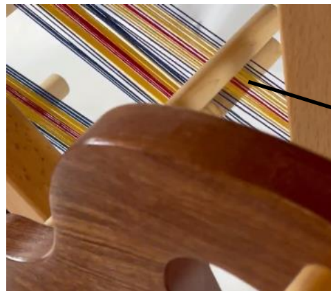
Two 'Fingers' Trap Unanchored Warp Yarns
