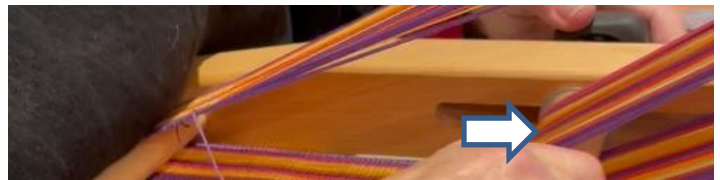
(Tensioner position in slot after re-tensioning)
