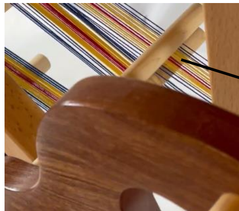
Two 'Fingers' Trap Unanchored Warp Yarns
